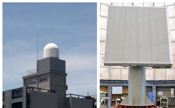
Fig. 1. Photographs of the PAR at Suita campus at Osaka University. The right photograph shows the 128-element antenna array of the PAR system inside the radar dome of the left photograph.
